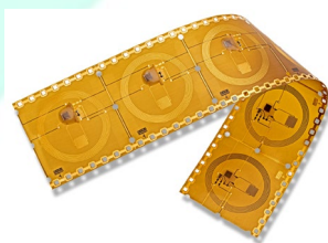
Linxens sensor for wound monitoring
